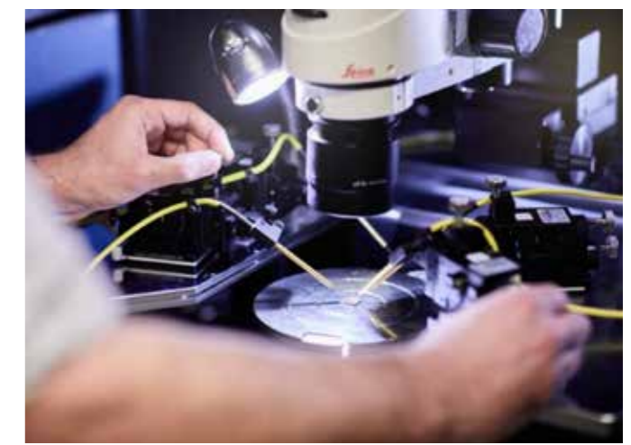
Electrical testing equipment in the Diamond Electronics Laboratory, showing variable temperature impedance spectroscopy (left) and a semiconductor characterisation system (right). In addition to measuring device parameters, these setups allow for the identification of novel carbon domains formed by the laser processing.
