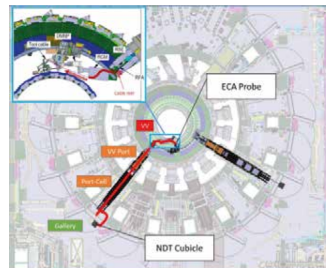
Figure 4 Layout of the cable routing between the control cubicle to the ECA probe
