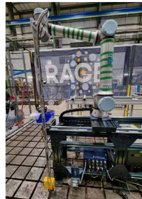
Experimental UR10e robot and aluminium payload setup
