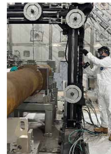
Checking cable wear during SAT
