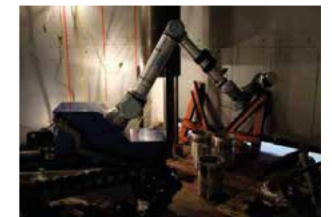
Inspections were also performed using the same sensors deployed on an ROV, in a mock-up environment representative of a nuclear decommissioning task.
